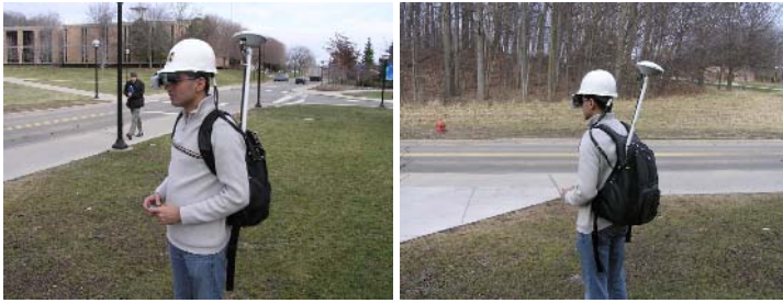
Fig. 4. AR Backpack Setup of UM-AR-GPS-ROVER
