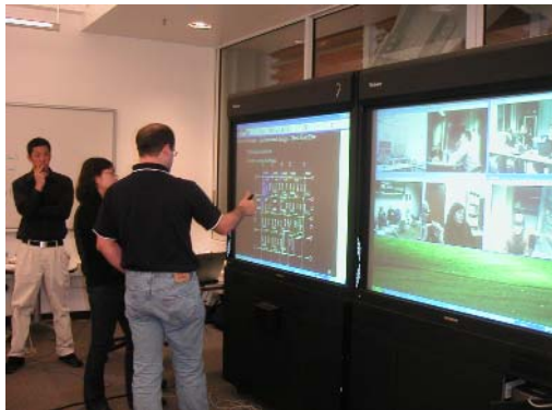
Fig. 3. Stanford Fishbowl™ ICT augmented workspace with VSee™. Left SmartBoard runs RECALL™ and NetMeeting with application sharing to allow Stanford and remote participants to sketch and annotate. Right SmartBoard runs eight VSee™ video streams.
